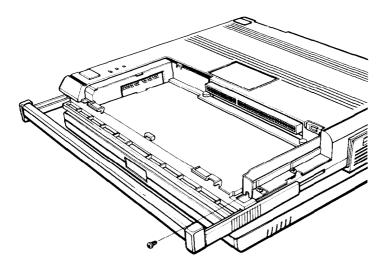
7. Insert the card from the back of the computer. Line up the connector on the card with the socket inside the expansion slot. Insert the connector directly into the socket. Secure the card with the screw you removed from the bracket.
